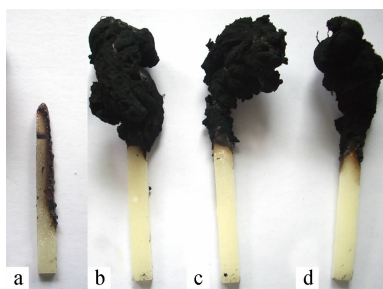
Fig. 3 Residue chars of FREP at the end of LOI test, EP (a), EP-EMFAPP10-8 (b), EP-EMFAPP20-8 (c) and EP-EMFAPP30-8 (d)
